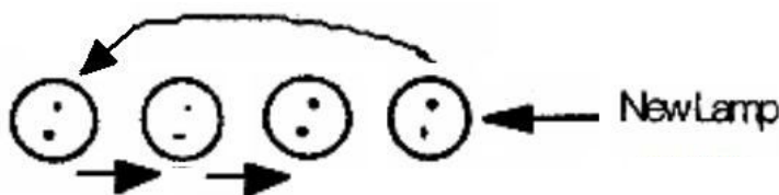
Fig. - Lamp replacement method.
